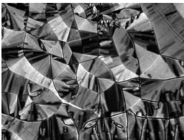
Fig. 5 Texture of the B_L phase (identified with the B_3 phase) in free standing film at T = 150 °C. The width of the picture is 300 \mu\text{m} .
